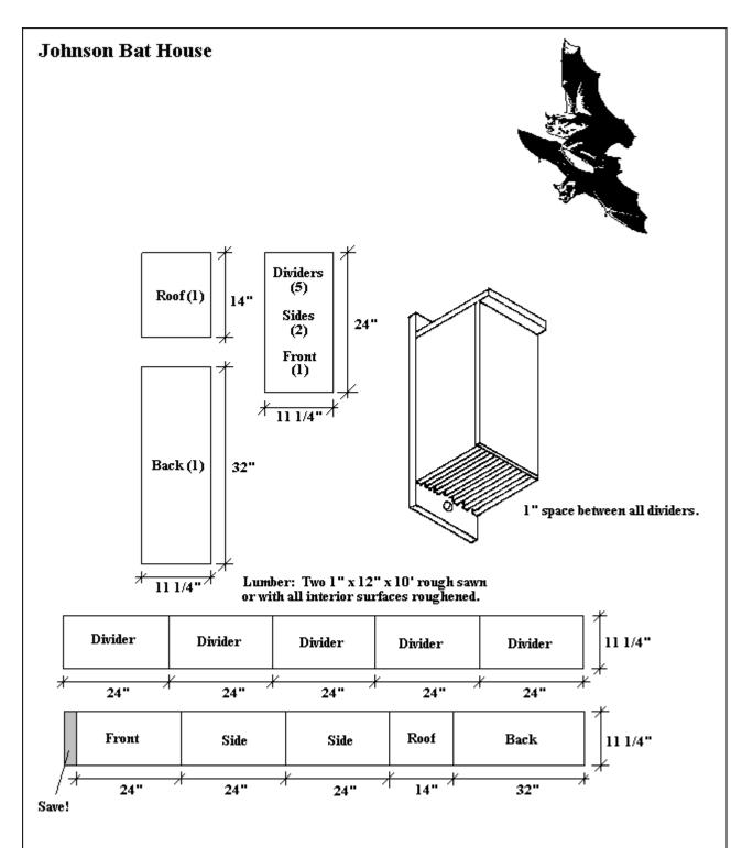
Note: All external seams and joints should be caulked if not tight fitting. Divider boards are spaced 1 inch apart.
